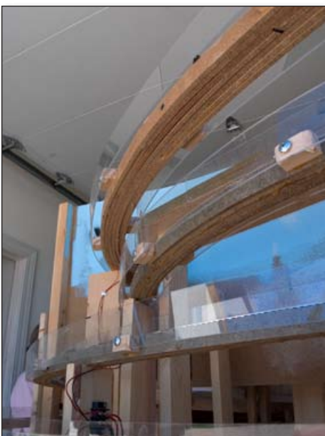
Spline roadbed and guard rails. Bob Sobol
