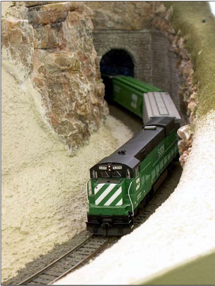
Leaning into the curve. Bill's spline roadbed automatically produces superelevation. Dave Zamzow
