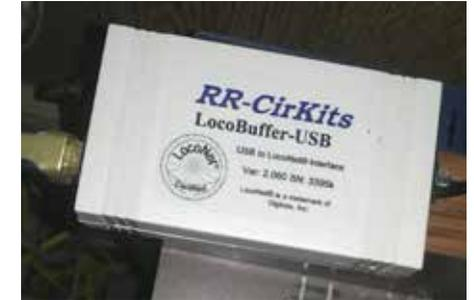
**Left:** NCE Power Pro systems have a DB9 serial port right on the front of the box; you just need to plug that into your computer, with a serial cable or a USB converter. **Right:** The LocoBuffer-USB needs to be acquired separately from RR-CirKits and this particular model already comes with a USB interface, and no converter is necessary.
